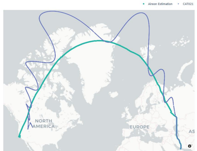
Fig. 9. Flight UAE51N on 2024-05-09 - Independent estimation of position (green) vs reported ADS-B data (purple).
