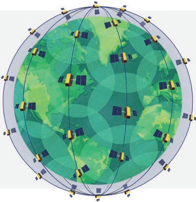
Aireon's space-based, global surveillance system is Automatic Dependent Surveillance-Broadcast (ADS-B) on a satellite. Instead of utilizing traditional radio towers on the ground, Aireon has redesigned them into flexible and highly-effective, space-grade receivers hosted on the global satellite constellation, Iridium NEXT. This allows for 100 percent air traffic surveillance using the same ADS-B avionics already installed on aircraft.
